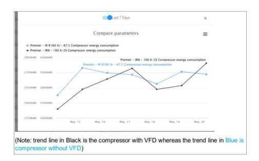
The fluctuating nature of the loads and therefore of the compressor energy consumption requires a smart tool to determine total energy consumption trends and identify optimisation opportunities.
